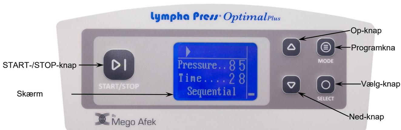
Figur 10 – Pumpens betjeningspanel
